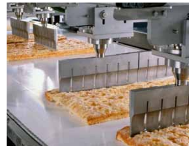
Ultraschall-Schneiden von Kuchen / ultra-sonic cutting of cake
