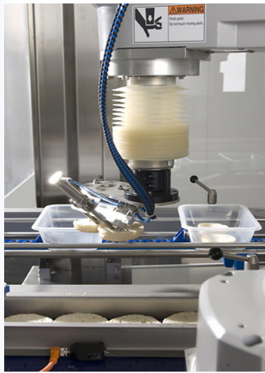
Scara-Roboter legt Brötchen in Schale scara robot places bun in tray
